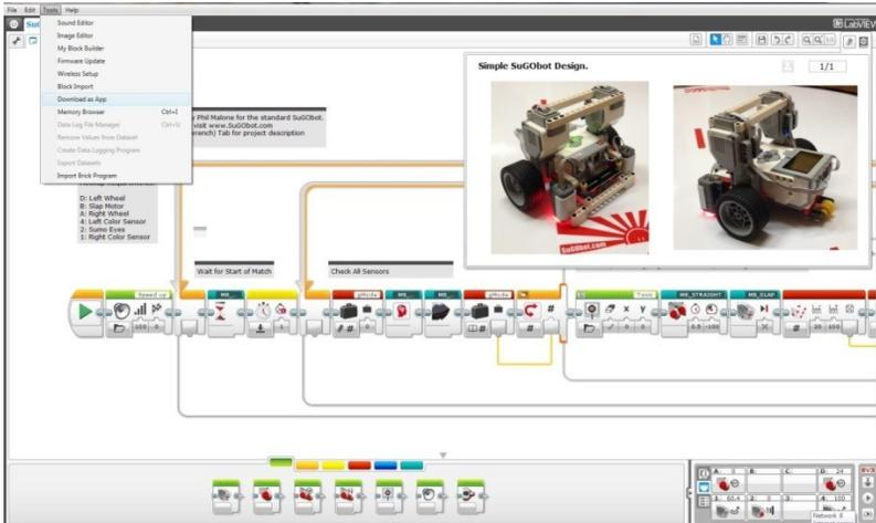
**BUT: DO NOT** load the SuGObot program onto the EV3 using the normal download button. Instead, create a SuGO app on your EV3 by using the “Tools/Download as App” menu item (shown above).
